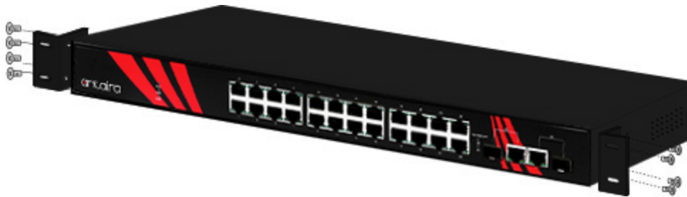
Figure 3.1 - Attach Mounting Plates with Screws
